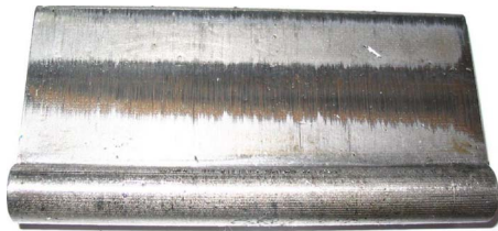
Fig. 13 Wear of the sliding vane
