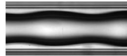
(c) Slug flow with a ring-shaped liquid film around a gas core
