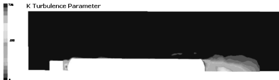
Fig. 12 k turbulence parameter on a horizontal plane 2 m above the road
