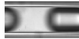
(b) Plug flow with two gas plugs separated by a short liquid slug
